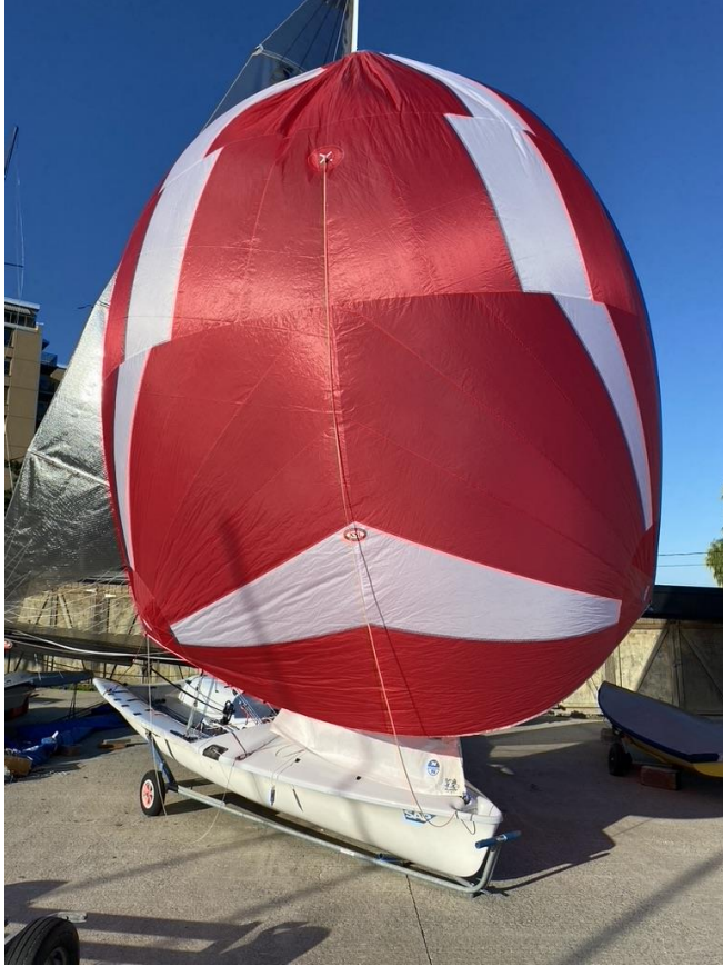
Figure 10: The First Prototype KSL 505 Spinnaker flying in very light air. We decided the retrieval patch (which was in the center of the sail) was too high, and lowered it after this image was taken. Image from Ali Meller.
