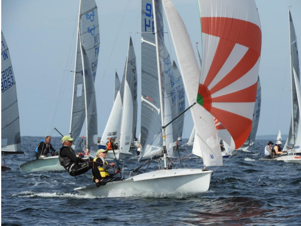
Figure 8: See the sharper radius vertical curve near the foot? This spinnaker design has also given up a fair vertical curve near the foot to support a little more foot round. Image from FB.
