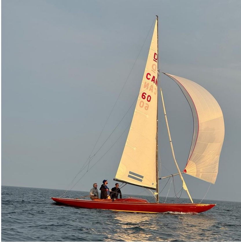
Figure 6: You can see the vertical discontinuity at the foot. This is to support a bit more foot round than the fair shape can. Image from Keven Piper.
