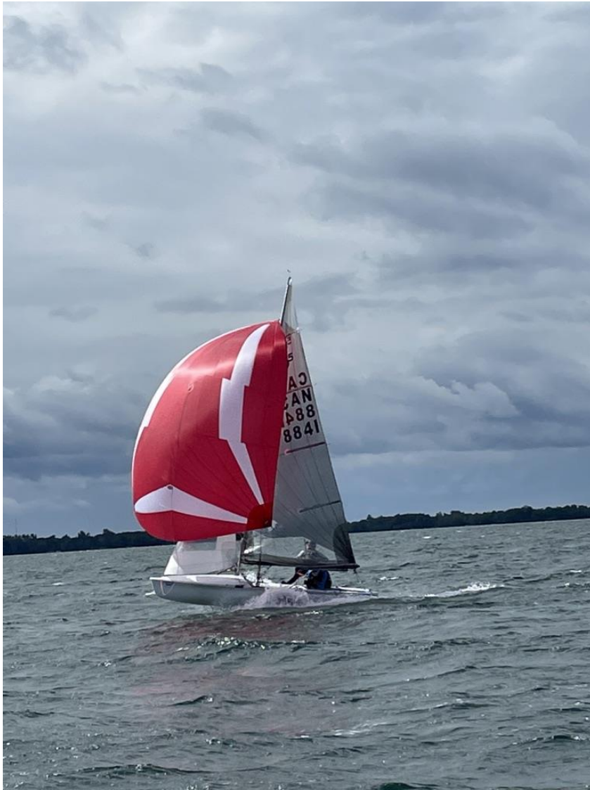
Figure 12: Note the smooth fair curves and no distortions at the foot. Even in a fresh breeze there is no stretching and changing of shape, as the warp threads line up with the loads on the spinnaker. We are still discussing if the spinnaker pole outboard end should have been slightly higher. Image from Sue Fraser.
