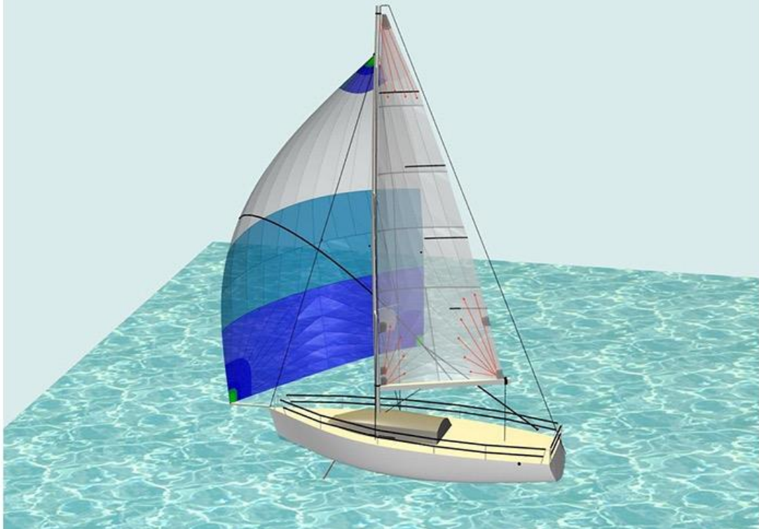
Figure 4: A Radial Quilt Cut Panel Layout on a Mainsail. No more crosscut panels. Image from a Keven Piper article.
