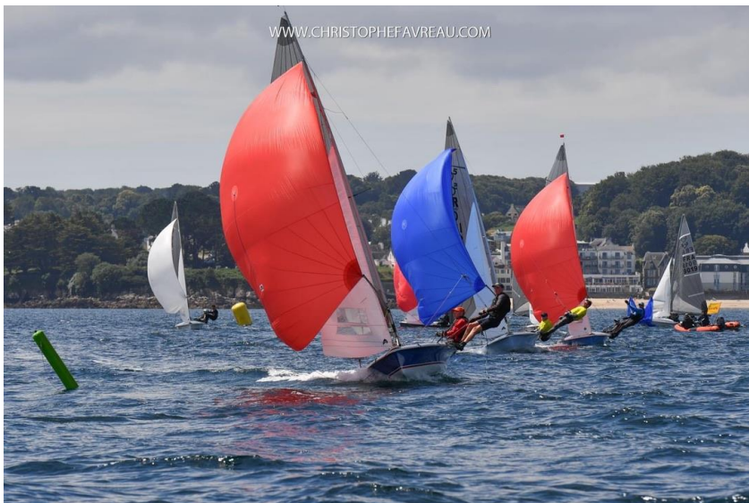
Figure 7: Both the nearer red spinnaker and the following blue spinnaker are showing an "in, then out, then in" to support more foot round. Image from Christophe Favreau via FB.
