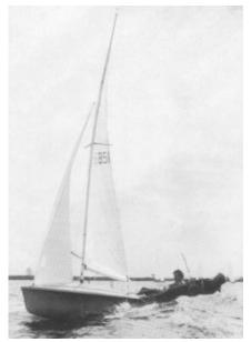
The jib luff is standing up straight but the mast appears to be bending to leeward which closes the slot between jib and main when it is very windy. Light air usually requires the mast rake to be a little less (more vertical), and it is an unfortunate trade-off to have to ease the jib halyard to attain sag - better to ease the shrouds.
