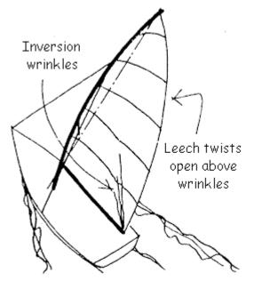
A mainsail which is 'inverted' (bent beyond its luff curve) develops large diagonal wrinkles that run roughly from clew to spreader (diagram), almost as though the back of the boom was bent off to leeward. This can provide a means of depowering without easing the sail too far outboard, retaining pointing ability.
