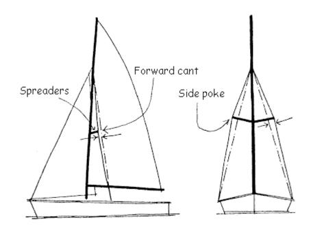
Having established, to a degree, how tension and spreader adjustment control mast bend, the important questions become, how does mast bend affect sail shape, and what do you want when?
