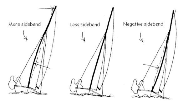
Longer spreaders, or more poke, tends to reduce side bend and can even force it negative. Shorter spreaders allow more side bend. Changes in tension work to increase or decrease the effect of the spreaders correspondingly - more tension and the spreaders do more work.
