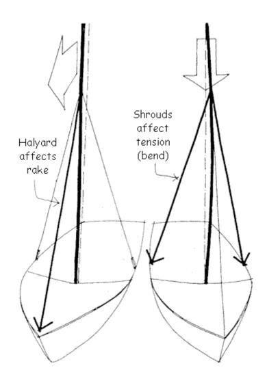
More forward cant on the spreaders, coupled with more shroud tension, causes less fore and aft mast bend. A reduction in either cant or tension will allow more fore and aft bend. If the spreaders are swept aft of a neutral position, increasing tension will induce more fore and aft bend.
