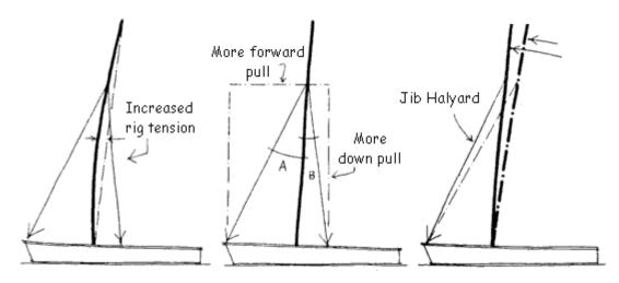
Jib halyard tension reduces rake and can also increase rig tension
